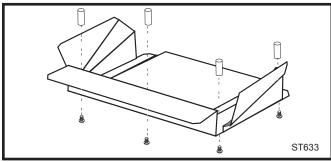
Fig. 14 Use four spacers to attach the bottom heat shield.
